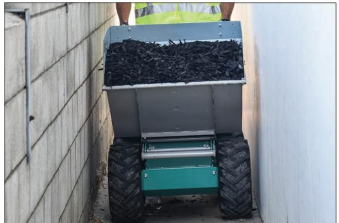
**Optional 7 ft<sup>3</sup> clip-on tub — TT7** — allows access through narrow 32-inch passageways.
