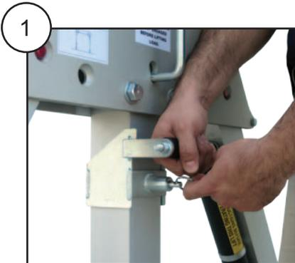
Adjust mast lifting handle with plunger pin to comfortable lifting position
