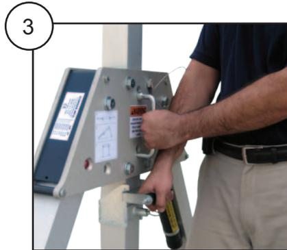
When lifting handle is next to frame, mast holes are aligned for locking pin
