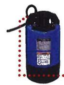
**NEW Dewatering pump LB-800A** features the Relay Unit (Level Sensor) which incorporates low voltage, stainless steel probes, epoxy and rubber encapsulated timing relay, that turns the unit off when liquid is not present. It saves energy and extends the life of the motor and bearings!
