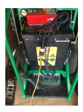
Connect the standard 110V plug directly to a power source. Preferably directly to the wall but if you are not close enough an extension cable will work. If using an extension cable, do not use anything over a 50ft long any smaller than a 12 gauge cord.
