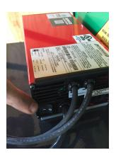
Once everything is connected, flip to switch from the "O" indicator to the "-" indicator. This should initiate the charger and the exhaust fan will begin to spin. Check the front panel to make sure you have an Orange LED light illuminated
