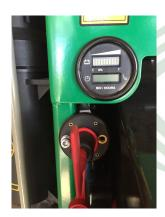
Chen ready to charge the machine, tun the key to the off position and remove the key.
