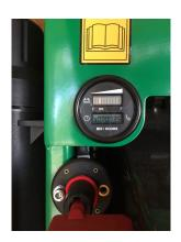
When the 100ECO battery indicator gets at or below 20% the battery indicator will turn from Green to Red. This indicates that it is time to charge the machine. Charging the machine if it is above 20% is ok, but overtime it will decrease the work-hour life of the battery.
