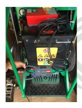
Plug the battery cable into the battery cable connector on the 110V charger.
