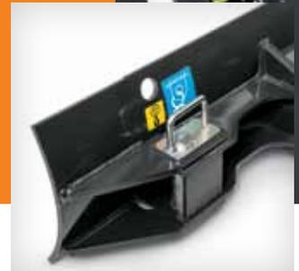
■ Redesigned blade extension pins allow you to effortlessly expand the width of the blade to match the track width on the ZX17U-5.
