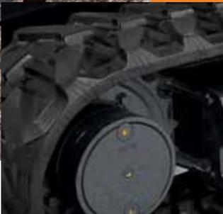
■ Unique steel cores within rubber tracks resist cracking, and large-diameter drive sprockets and track idlers make for a rock-solid undercarriage.
