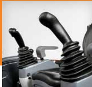
■ Ergonomically correct short-throw pilot levers provide smooth, precise control with less effort.
