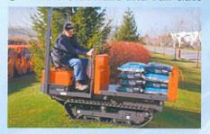
Not only the tailgate, but also the sidewalls on both sides of the bed are hinged to permit being either raised or lowered to efficiently accommodate the specific load to be transported. In addition, the sidewalls and the tailgate are removable to permit the KC120HC to be used as a flat bed carrier.
