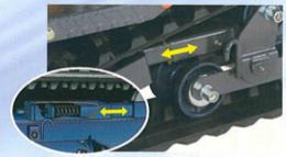
The built-in springs fitted to the tension adjusters absorb shock in order to help prevent damage to the rubber crawlers.
