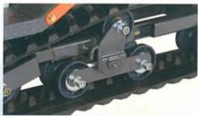
Even over undulating terrain, the bogie-type under rollers contribute to more stable travel.
