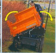
To more efficiently handle operations in confined spaces, the bed for the KC120HC can be dumped in three directions - forward, left, and right.
