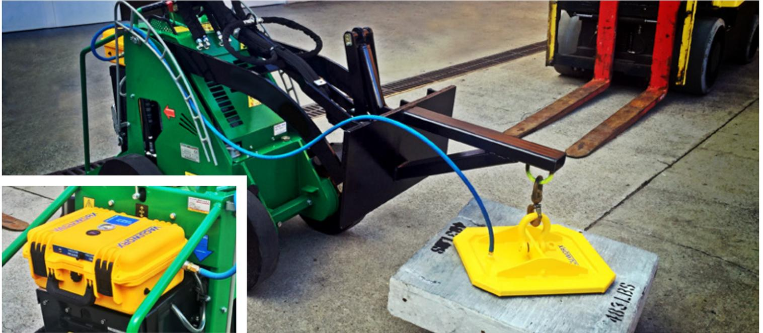
**THE PS 1 PORTABLE VACUUM LIFTING SYSTEM** is the perfect solution for smaller lifting challenges that come up daily on jobsites or in the shop. Designed for interior and exterior applications, the patent pending PS 1 can lift up to 1,500 lb (0.7 tonne) and is a great companion to small equipment such as skid steers, electric skid steers, mini electric excavators, forklifts and small cranes.
