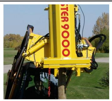
**Hydraulic Tilt** - Tilt 20 degrees left and right. Keep posts aligned when operating on hills.
