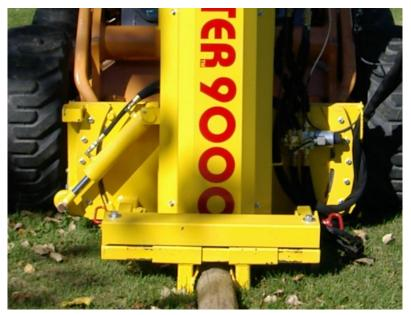
**Post Grapple** - Can be added to any model for a one-man operation. Grab the post off the ground, load it into the machine, and drive it in the ground without leaving the skid-steer seat.
