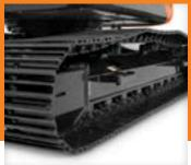
With large idlers, rollers, and strutted links, the sealed and lubricated undercarriage delivers long, reliable performance.
