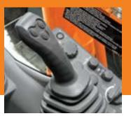
Ergonomically correct shortthrow pilot levers provide smooth, precise fingertip control with less movement or effort.
