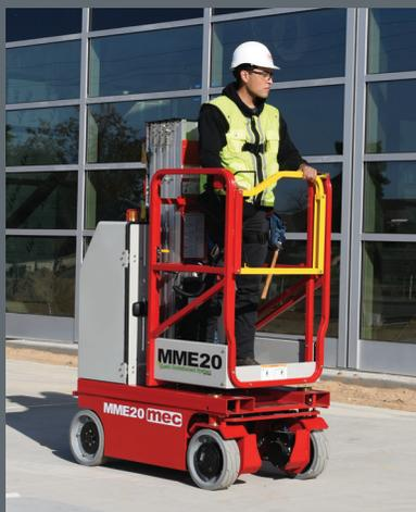
**Important** - MEC mast lifts must be on a hard level surface while elevated.
