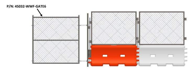
**Step 5:** Position P/N 45032-WWF-GATE6, Gate in front of the Attachment Frame and assemble it by aligning the female clip on the Gate to the male hinge clip on the Attachment Frame.
