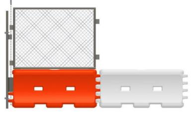
**Step 5:** Position the 2nd Fence Panel on the Water-Wall, making sure that the flat plate on the fence frame is positioned on top of the Water-Wall. Assemble by aligning the rectangular slots on both the fence frames and inserting the T-pin through the slots which also goes through the holes on the knuckles of the Water-Wall.
