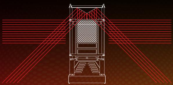
THE UPPER, REFLECTIVE CONE DIRECTS INFRARED HEAT TO THE SURFACE BELOW WHILE MAINTAINING A O" CLEARANCE TO COMBUSTIBLES!
