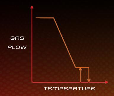
THERMOSTATICALLY CONTROLLED, MODULATING VALVE DECREASES OR INCREASES THE AMOUNT OF GAS SUPPLY TO MAINTAIN THE DESIRED TEMPERATURE
