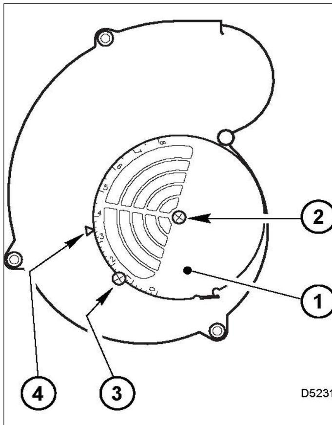
**C)** The final position of the air adjustment plate will vary on each installation. Use instruments to establish the proper settings for maximum CO<sub>2</sub> and a smoke reading of zero.
