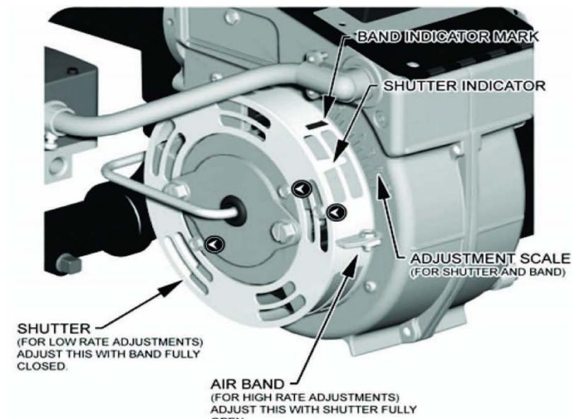
**WARNING: LACK OF COMBUSTION AIR CAN CAUSE A DIRTY FIRE, ODOURS IN ENCLOSED SPACES, AND BACKDRAFTING, POTENTIALLY RESULTING IN NAUSEA OR ASPHYXIATION OF THE OCCUPANTS.**
