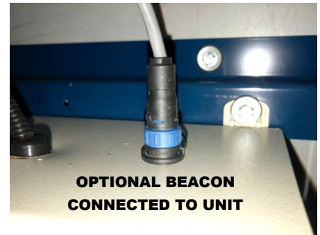
BEACON CONNECTOR PROVIDED AT TOP OF CONTROL PANEL
