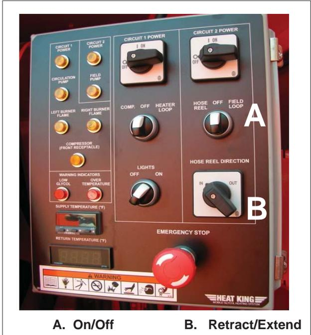
Fig. 33 REAR CONTROL PANEL. HK500 shown above, HK150/300 below.
