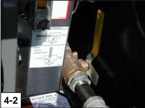
4. Turn the PUMP Switch ON to continue filling and turn OFF when the HTF level is between MIN and MAX lines on the Sight Gauge Decal. Place the 3-Way Valve #2 to the NORMAL position. Replace the Hose End Cap and stow the Fill Hose neatly under the Hose Reel or Burner.
