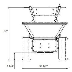
DriveElectricElectric tension24VPower1000 WClimbing abilityMax. 40 %Revolutions per minute2200 RPM
