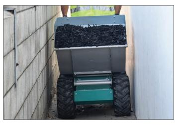
**Optional 7 ft³ clip-on tub — TT7** — allows access through narrow 32-inch passageways.
