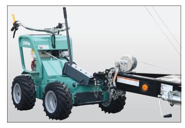
**TuffTruk 2-Inch Towing Hitch** — **TBH** — offers various height positions for different size trailers.
