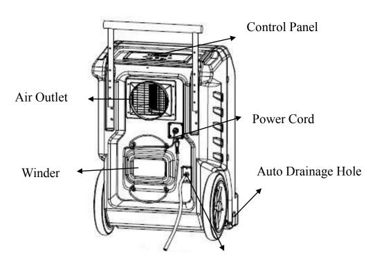
Water Hose Connector (Manual Drainage)
