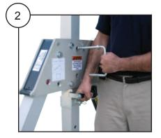
Lift mast and remove quick-action mast locking pin – no bolts!
