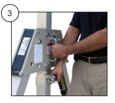
When lifting handle is next to frame, mast holes are aligned for locking pin
