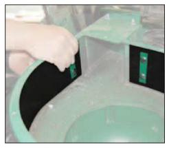
**Optional liner sleeve** protects housing in sandy conditions (Part No. 891134) and new Shredder Kit reduces dry leaves up to 12:1 (Part No. 891153)
