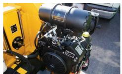
25 HP (18.6 KW) EFI ENGINE performs well during cold-weather starts, reduces occurrence of engine flooding and provides improved fuel economy over comparable carbureted gas engines.
