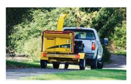
THE WIDE AXLE offers an ample footprint at the axle for side-to-side stability; additionally enhances transportability and visibility while backing up.
