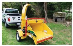
THE LARGE INFEED OPENING 6" x 8" (15.2 cm x 20.3 cm) makes feeding irregular material easier and decreases the amount of saw cuts needed prior to feeding the chipper.
