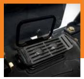
Swing boom and foldable travel pedals on the ZX26U-5 are positioned where they're easy to operate, yet allow plenty of foot room.
