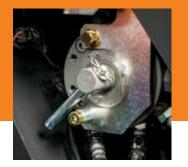
Go from backhoe- to excavator-style controls with just a twist of your wrist. Control-pattern selector valve is conveniently located in a compartment beneath the seat and includes a sight glass that displays the selected pattern.
