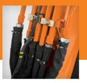
Steel hydraulic lines are clamped securely, and wearresistant hoses are protected with Cordura<sup>®</sup> covering.
