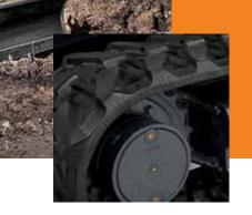
Unique steel cores within rubber tracks resist cracking, and large-diameter drive sprockets and track idlers make for a rock-solid undercarriage.
