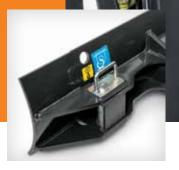
Redesigned blade extension pins allow you to effortlessly expand the width of the blade to match the track width on the ZXI7U-5.
