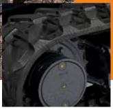
■ Unique steel cores within rubber tracks resist cracking, and large-diameter drive sprockets and track idlers make for a rock-solid undercarriage.
