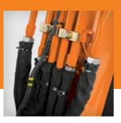
■ Steel hydraulic lines are clamped securely, and wear-resistant hoses are protected with Cordura® covering.
