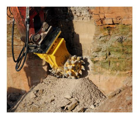
The drum cutting technology used allows **accurate removal of material** in tunnels and trenches, and from any other kind of rock or concrete surface.
