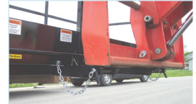
Fork Pocket Safety pin installed
