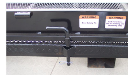
Door Safety Pin (Locked Position)
