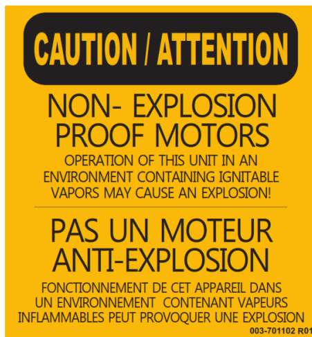
Figure 2-2: DECAL CAUTION NON-EXPLOSION PROOF
