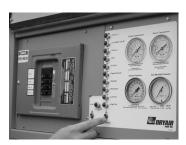
Figure 21 -water heater on/off toggle switch
