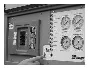
Figure 20 -pump on/off toggle switch
