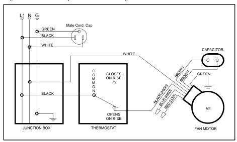
Figure 40 – electrical - portable heat exchanger – 600 model
