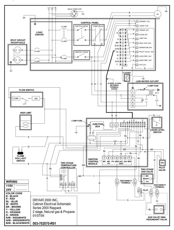
Figure 40 – electrical - portable heat exchanger – 80 & 200 model
