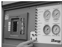
Figure 16 - turning on water heater toggle switch
