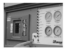
Figure 15 - turning on breakers switches and pump toggle switch
