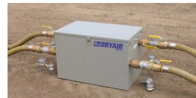
Figure 3-5 Mixing / Booster Pump
