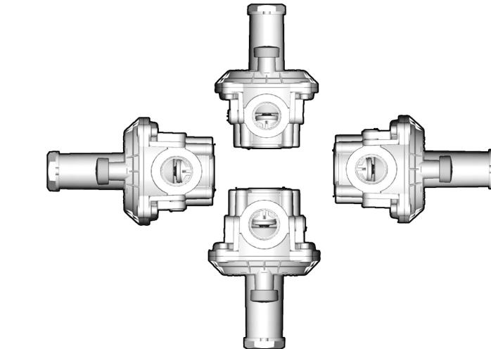
In case of upside-down installation the setting value of the spring changes and the regulation pressure must be readjusted as indicated in paragraph 3 on page 2.
